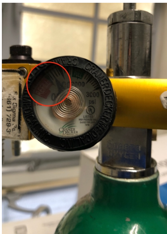
Photo 8. Oxygen tank with pressure below 1,000 psi (photographed on July 16, 2021).
