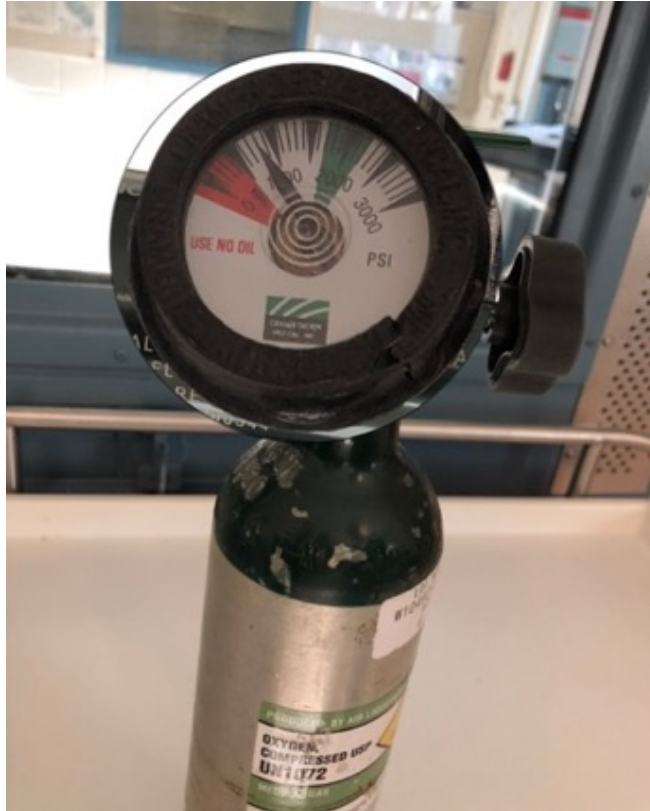
Photo 11. EMRB oxygen tank pressure at 800 psi (photographed on March 5, 2021).
