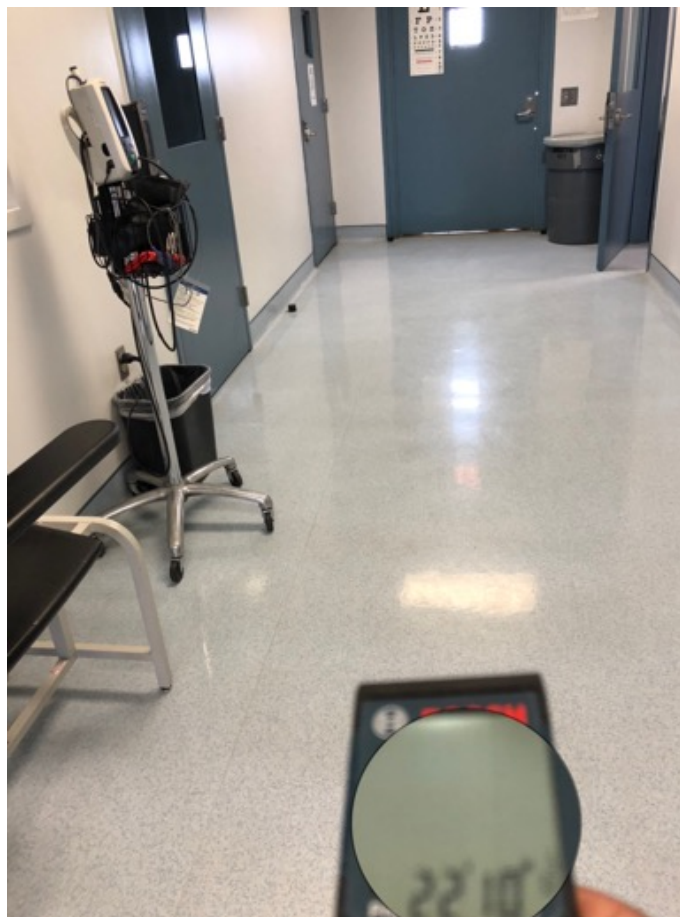
Photo 10. The Snellen eye chart was placed at an improper distance of 22 feet and 10 inches. The proper distance is 20 feet (photographed on March 3, 2021).
