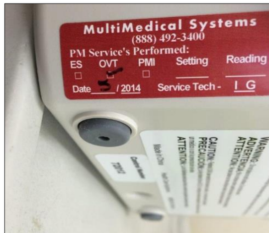
Figure 4: Nebulization unit with expired calibration
