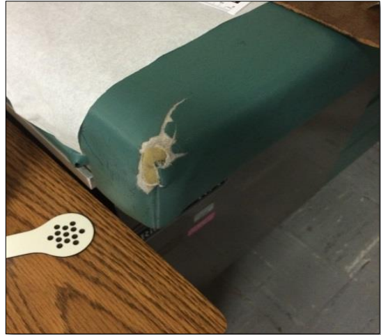
Figure 3: Worn vinyl on exam table
